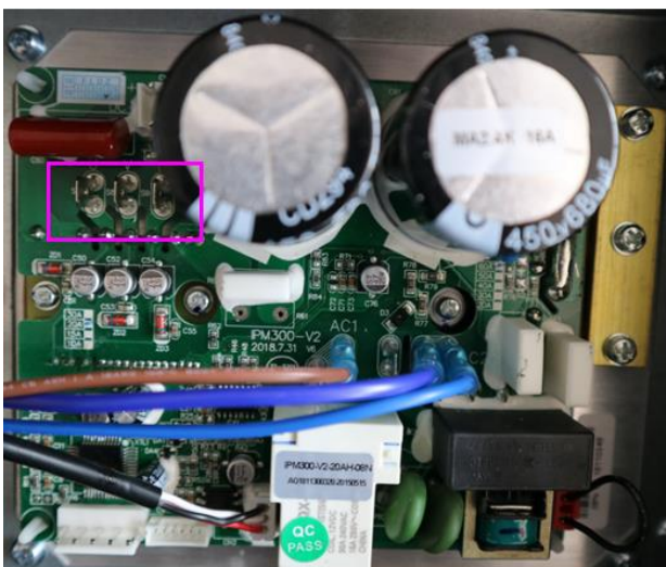
Inverter Board( Single Phase)
