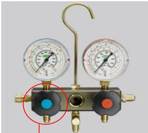
Low pressure gauge valve
